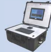
Figure 5: The PL100-GEO battery-operated field portable LIBS instrument (Applied Spectra, Inc.)
