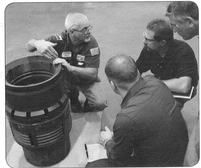
Inspection of SS-15 BigBore II-H casing hanger
