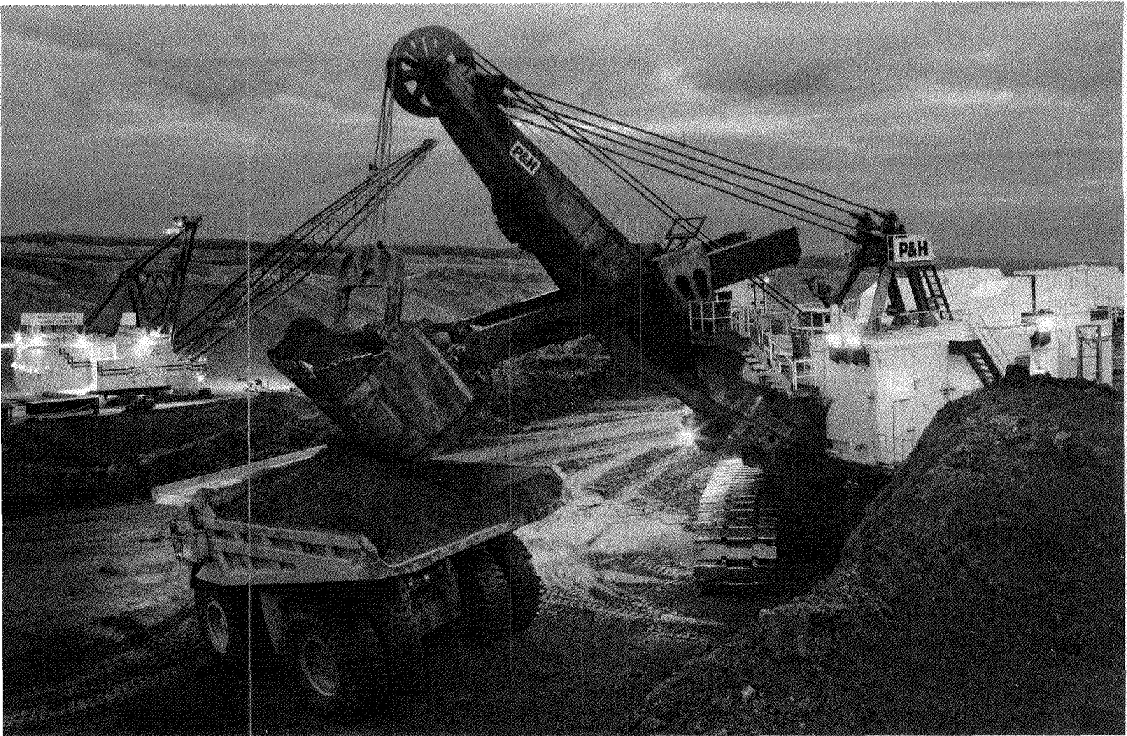
A truck/shovel operation works into the night to uncover coal at the Mississippi Lignite Mining Company's Red Hills Mine in Mississippi.
