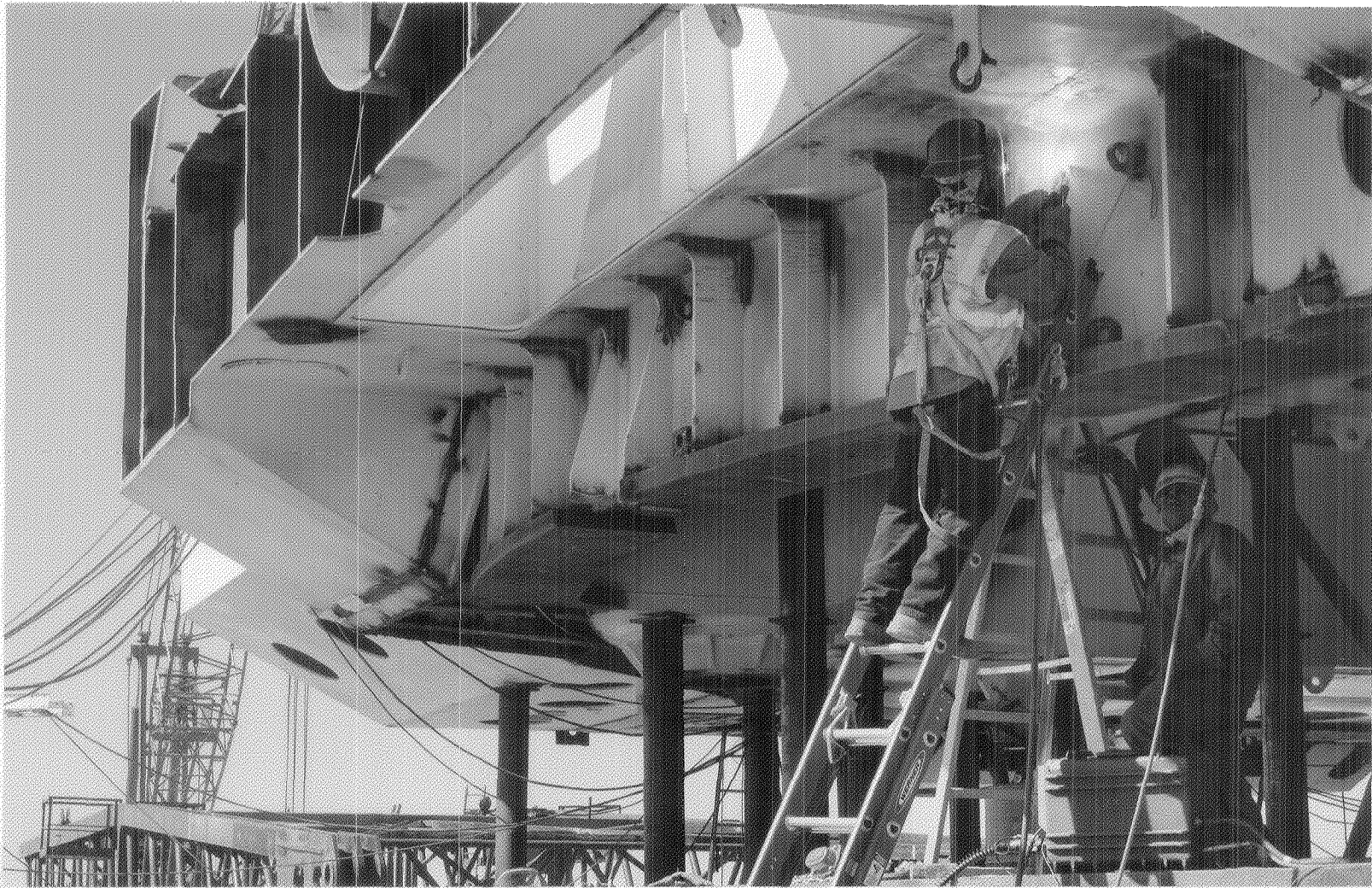
Much of the development work at the new Liberty Mine in Mississippi involves assembling mining equipment, such as this dragline that will eventually be used to remove overburden.
