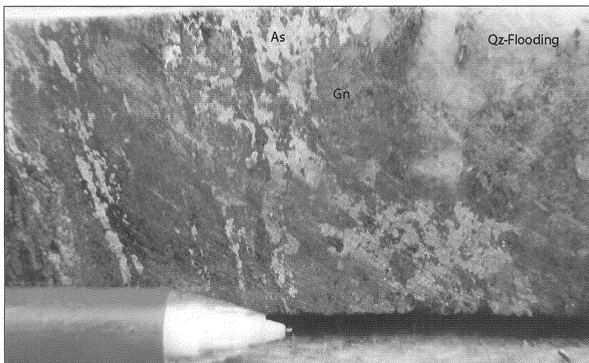
Picture 19: Drillhole NO-03-018A showing quartzflooding, grunerite alteration and arsenopyrite. This interval returned 1.63 g/t Au over 1.00 m (#746813).
