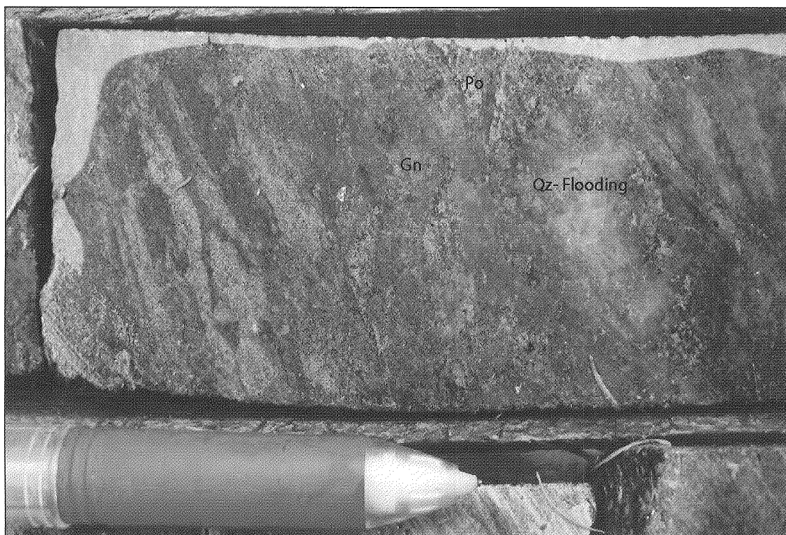
Picture 20: Drillhole NO-03-011B showing quartz flooding (vein?), grunerite and pyrrhotite that returned 1.99 g/t Au over 0.80 m (Sample 209701).
