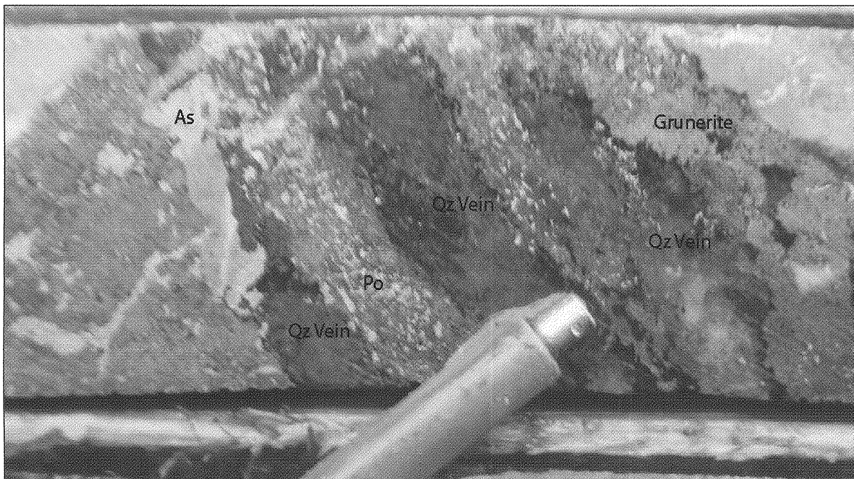
Picture 18: Drillhole NO-03-08B showing quartz veins in a grunerite-rich banded iron formation that also present evidence of sulphide remobilization. This interval has returned values of 2.94 g/t Au over 0.65 m (sample 209619).
