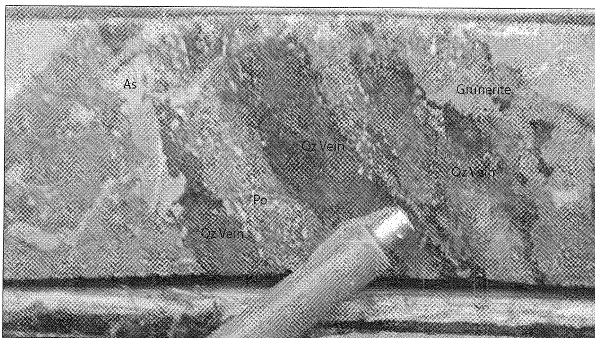
Picture 18: Drillhole NO-03-08B showing quartz veins in a grunerite-rich banded iron formation that also present evidence of sulphide remobilization. This interval has returned values of 2.94 g/t Au over 0.65 m (sample 209619).
