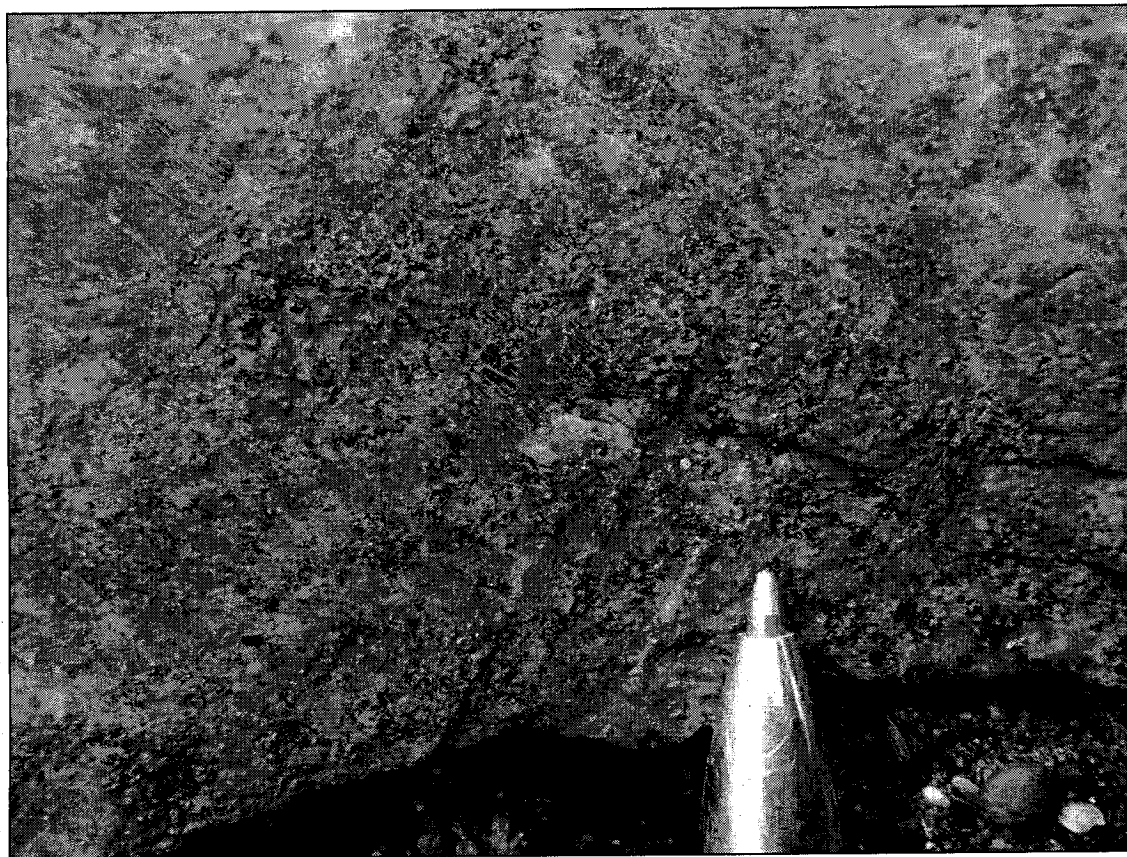
Picture 2: Garnet and chlorite alteration from channel PAU-2010-R-072 (Sample 202057) in trench PAU-2010-TR-066.
