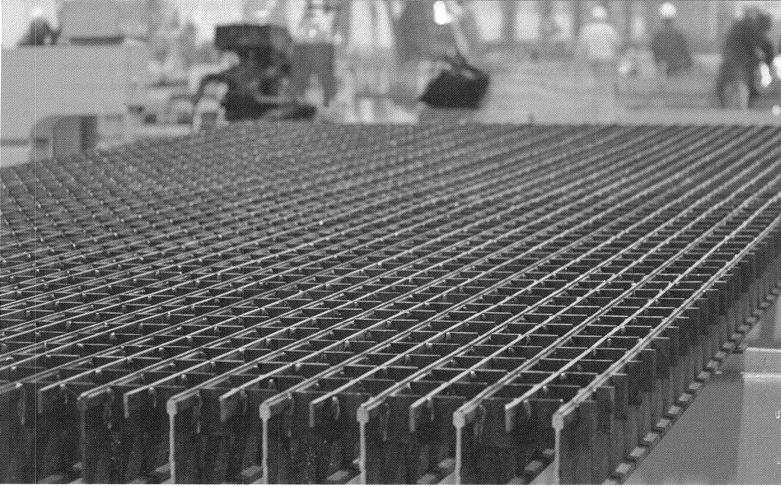
INNOVATIVE STEEL GRID BRIDGE DECKING MANUFACTURED AT L.B. FOSTER'S BEDFORD, PA FACILITY ▼
