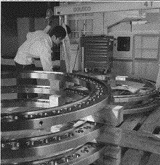
Tao Zhang, operator for green turning, inspects an ultra-large wind bearing at the new facility in Xiangtan, China.
