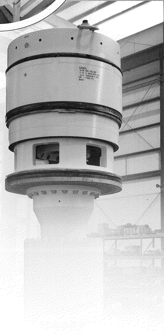
CSO Diverter Cartridge in Final Assembly
