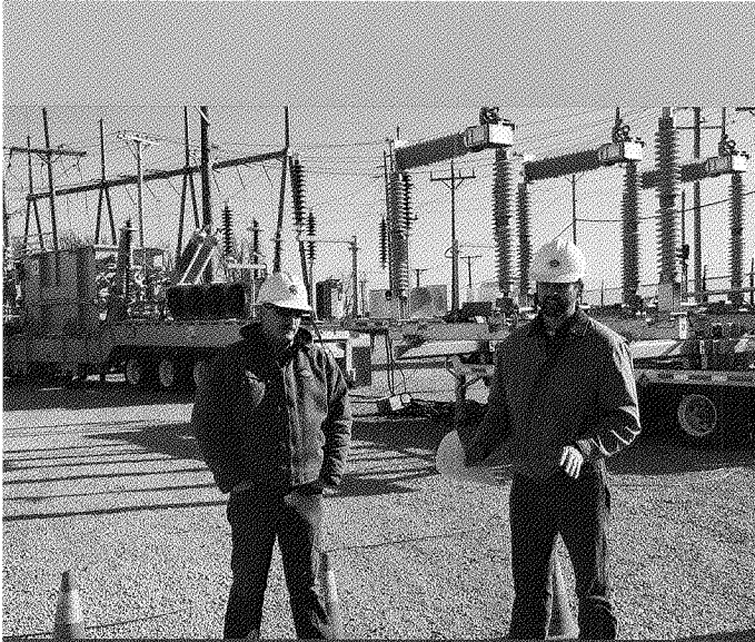
An additional portable substation, designed and engineered to fit Empire's specific needs, was acquired and readied for service this past year. Basically a complete substation on wheels, it can keep the lights on for customers during routine maintenance or an unexpected outage. David, Substation Maintenance, and Sam, Engineering and Line Services.
