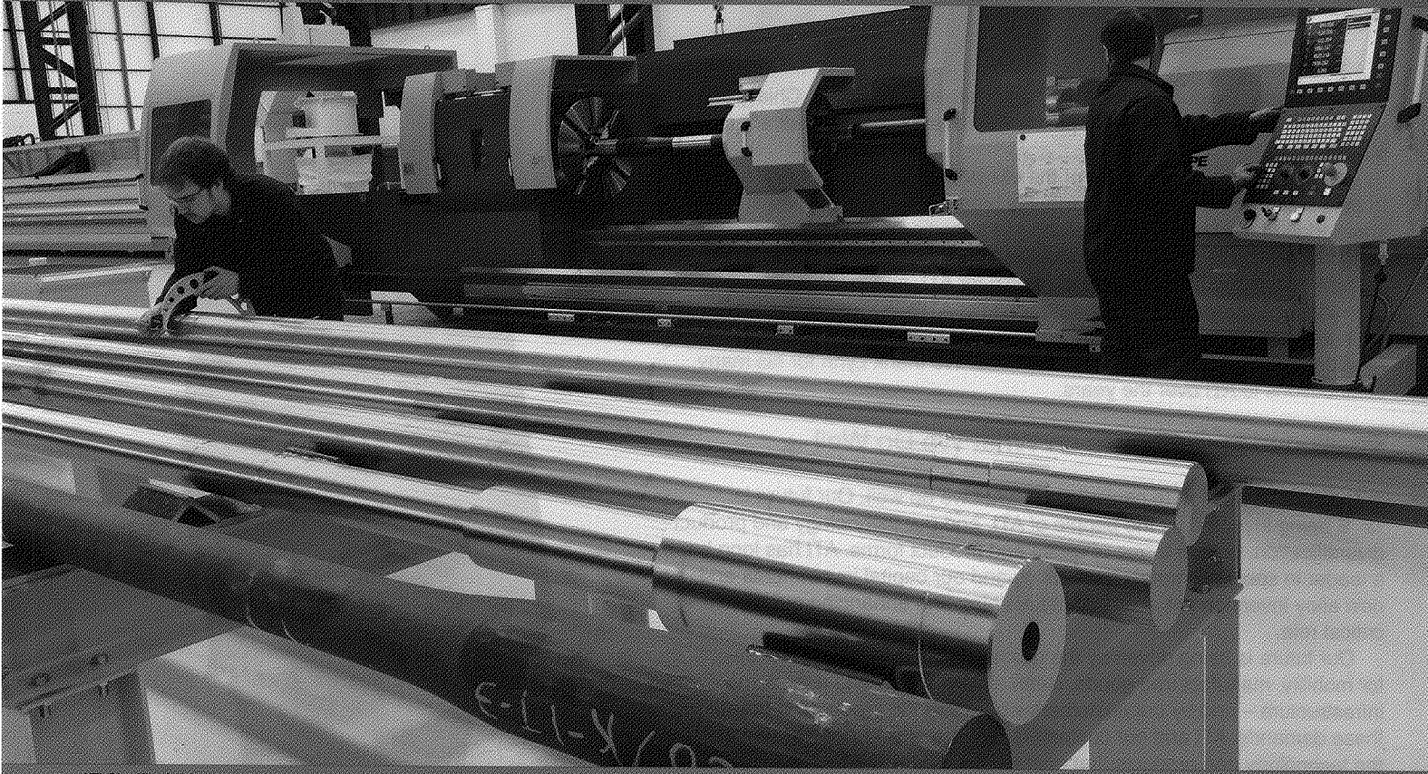
ATI Sheffield, Precision Machinists Matthew Hill (l) and Martyn Webb (r) working at a computer-numerically-controlled (CNC) lathe in the Company's recently-completed Precision Machining Facility. On the rack in front of the lathe are an ATI 718™ alloy rotary steerable shaft net-shape forging, pre- and post machining, with several ATI Datalloy 2® Drill Collars behind.
