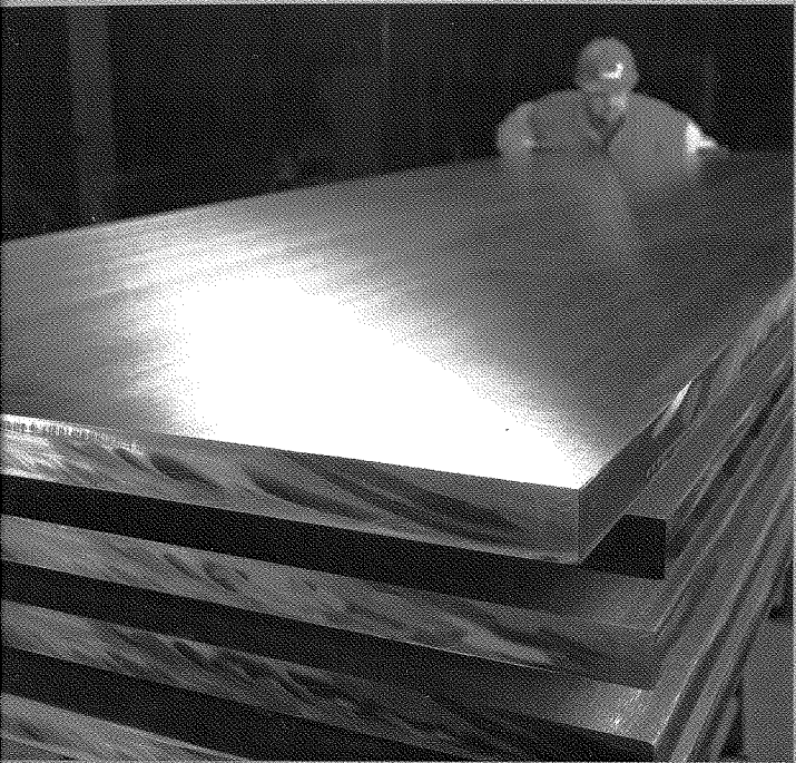
ATI 425® Alloy titanium plate undergoes final inspection after grinding by ATI Precision Finishing to assure proper surface and flatness before shipping to Aerospace and Defense customers.
