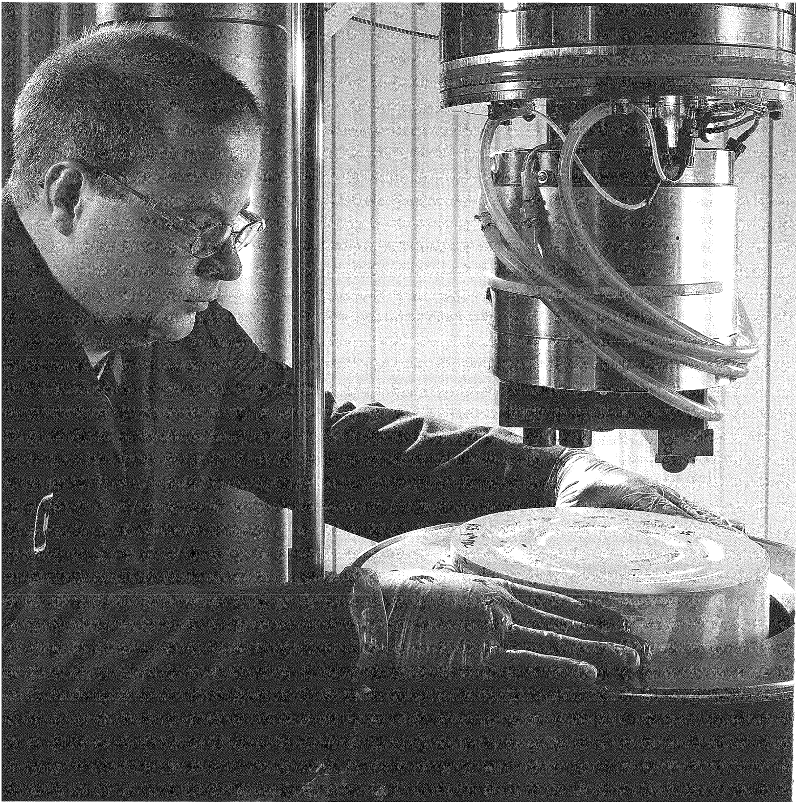
Designing for Faster Drilling (above) Engineering tests in the laboratory translate to better drilling performance in the well. Technician Ryan Meng prepares to test a polycrystalline diamond compact (PDC) cutter design on a sample rock formation at the Smith Bits Engineering Center in Houston, Texas, USA. The results are used to simulate the drilling mechanisms and optimize the design of the bit.
