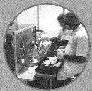
100 percent electrostatic hole detection being carried out at the production facility in India.
