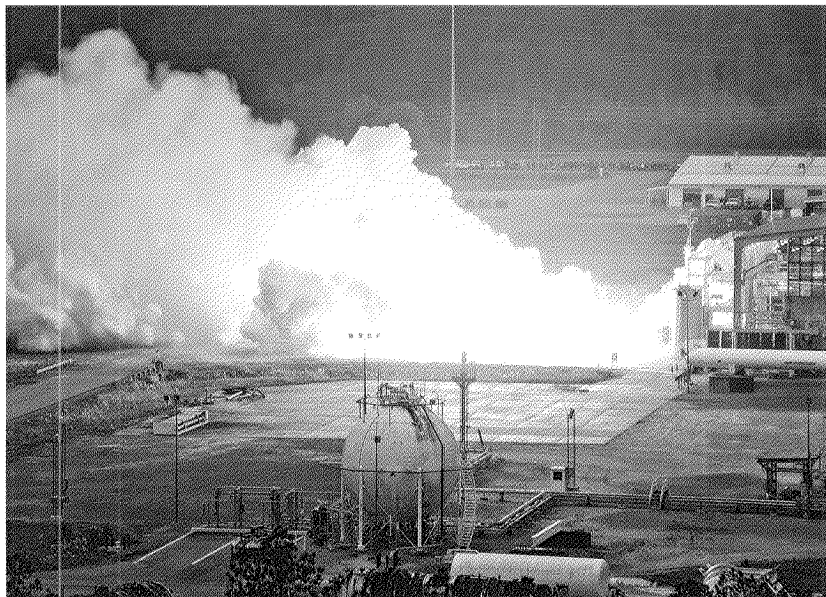
Initial testing of the AJ26 rocket engines that will power the first stage of our first Taurus II launcher was completed in 2010 at NASA's Stennis Space Center.
