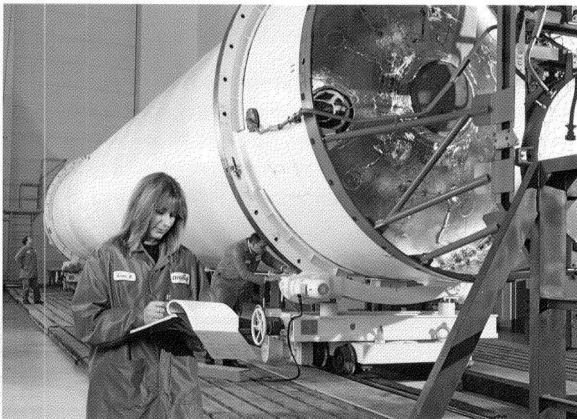
Last year saw substantial progress in the development of our Taurus II medium-class rocket. The first 90-foot long stage one core structure (left), was designed and built in Ukraine and arrived at Wallops Island, Virginia in November 2010.
