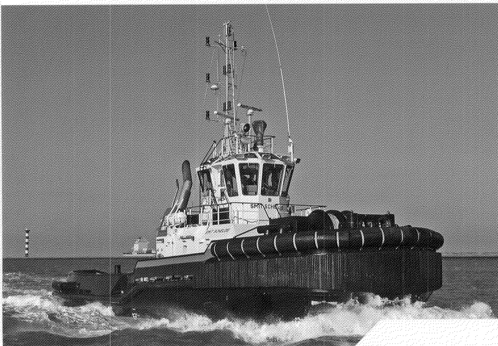
2810 ASD harbour tug "Smit Schelde" is part of the SMIT Harbour towing fleet in the port of Rotterdam.
