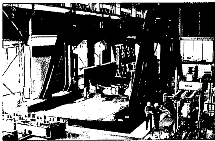
▲Railway Structure Loading Test System
