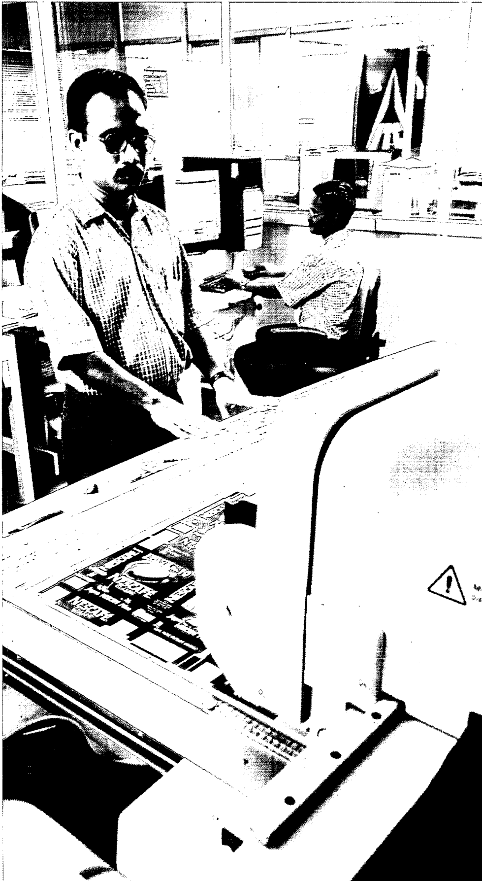
The Kongsberg enables quick samples to be cut from die-CAD The BMA (right) offers hot foil stamping, hologram
