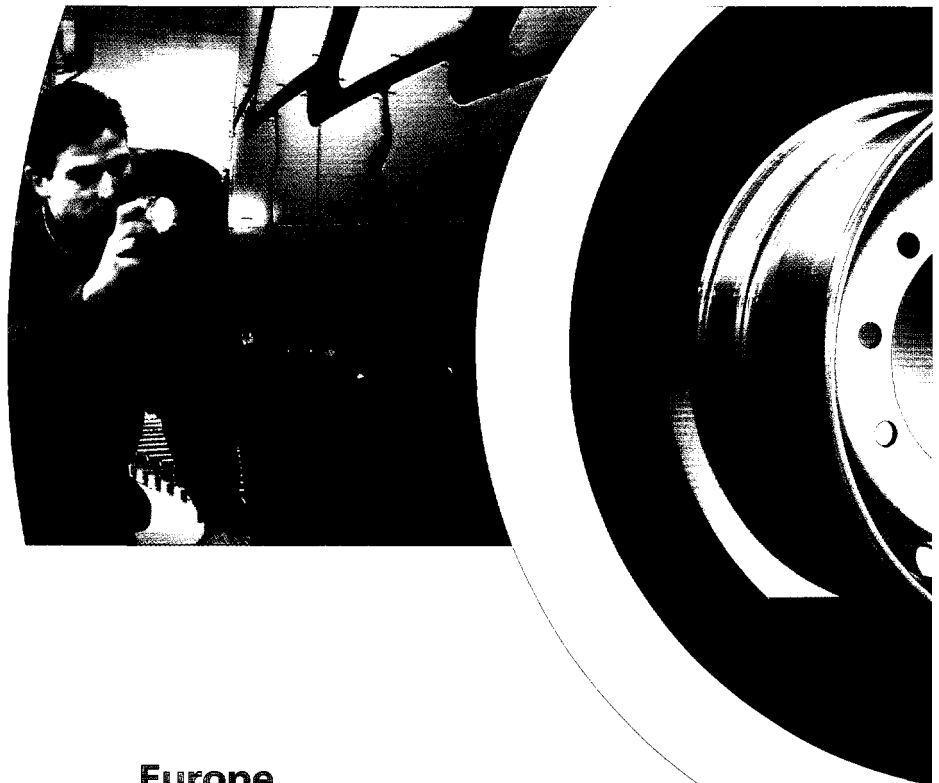
Michelin introduced its new giant tire, the 56/80 R 63 XDR at the 2004 MINExpo at Las Vegas. As the newest arrival to the line aimed at oversized dumpers, this tire measures 4 meters in diameter, is 1.425 meters wide and weighs 4.9 metric tons.
