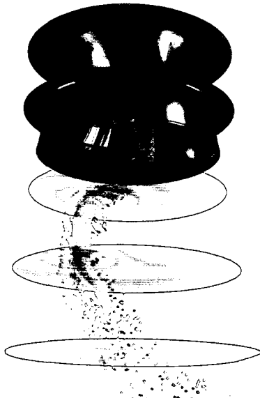
CFD simulation of a draft tube vortex at part load.
