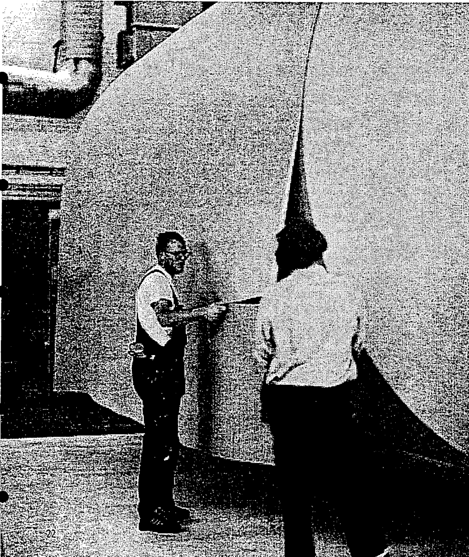
Pontus Andersson and Tapio Livanainen (back to camera) taking samples from a cylinder/tambur, which will be submitted for quality control at the plant's laboratory. A tambur weighs some 50 tonnes and can measure up to about 4 m across.
