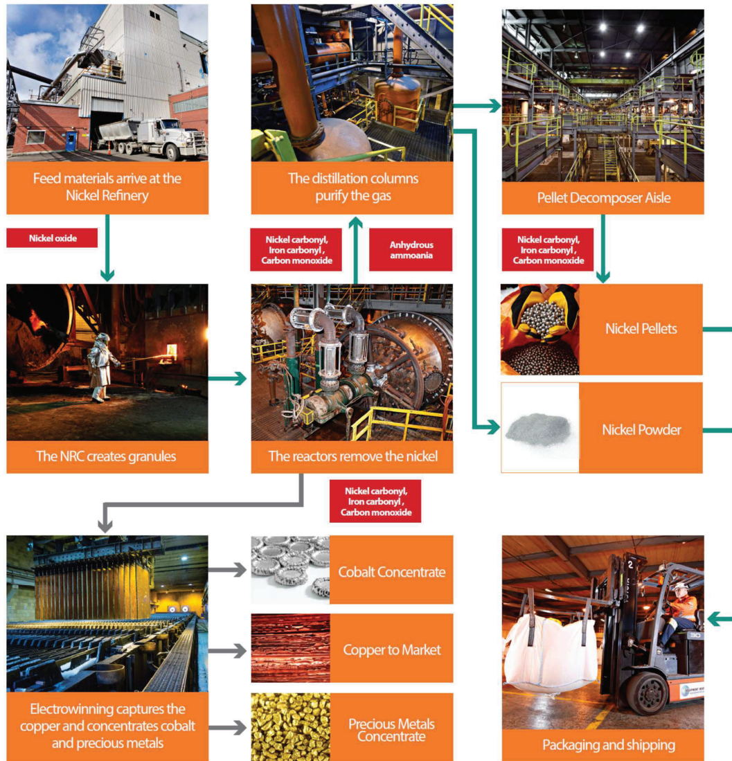
Figure 14-5: Schematic Flowsheet, Copper Cliff Nickel Refinery
