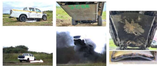
STANAG AEP55 Testing of ABBS Shockwave Mitigating, Energy Absorbing, Composite Reinforced Sandwich Belly Plate on a Toyota Hilux over a 4kg buried under belly charge, resulting in 4.5-metre jump height and 125mm (5") indentation of the Faceplate and the same 175mm (7") back face deformation.
