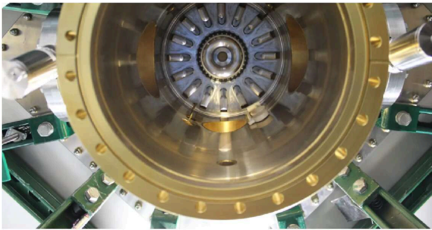
Focus Fusion Electrodes View From The Bottom, Through The Vacuum Chamber (Not Yet Assembled)
