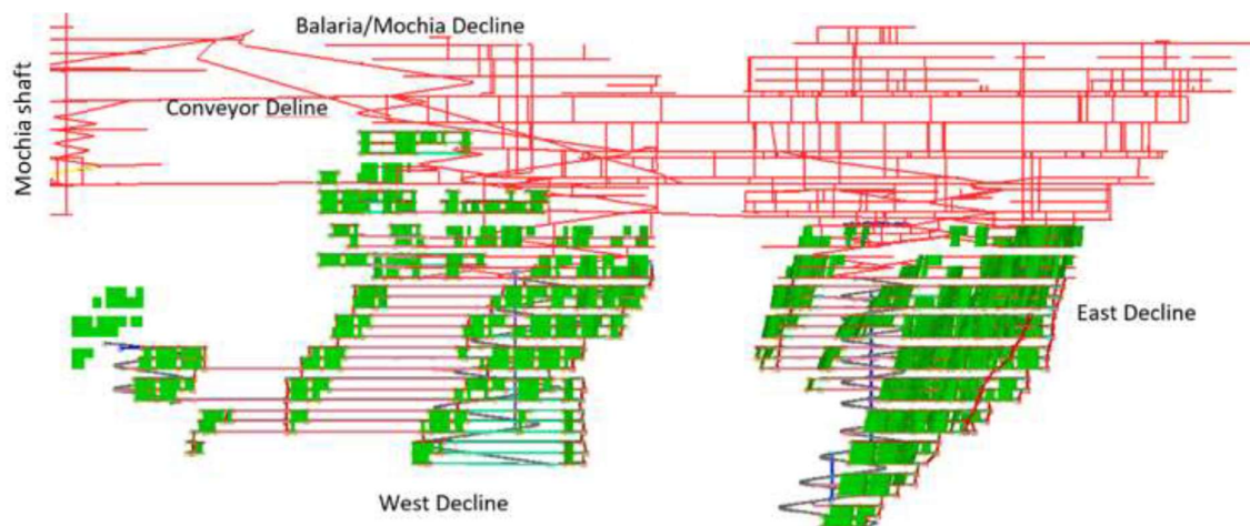
Figure 27: Section view of the main declines for Balaria Mine
