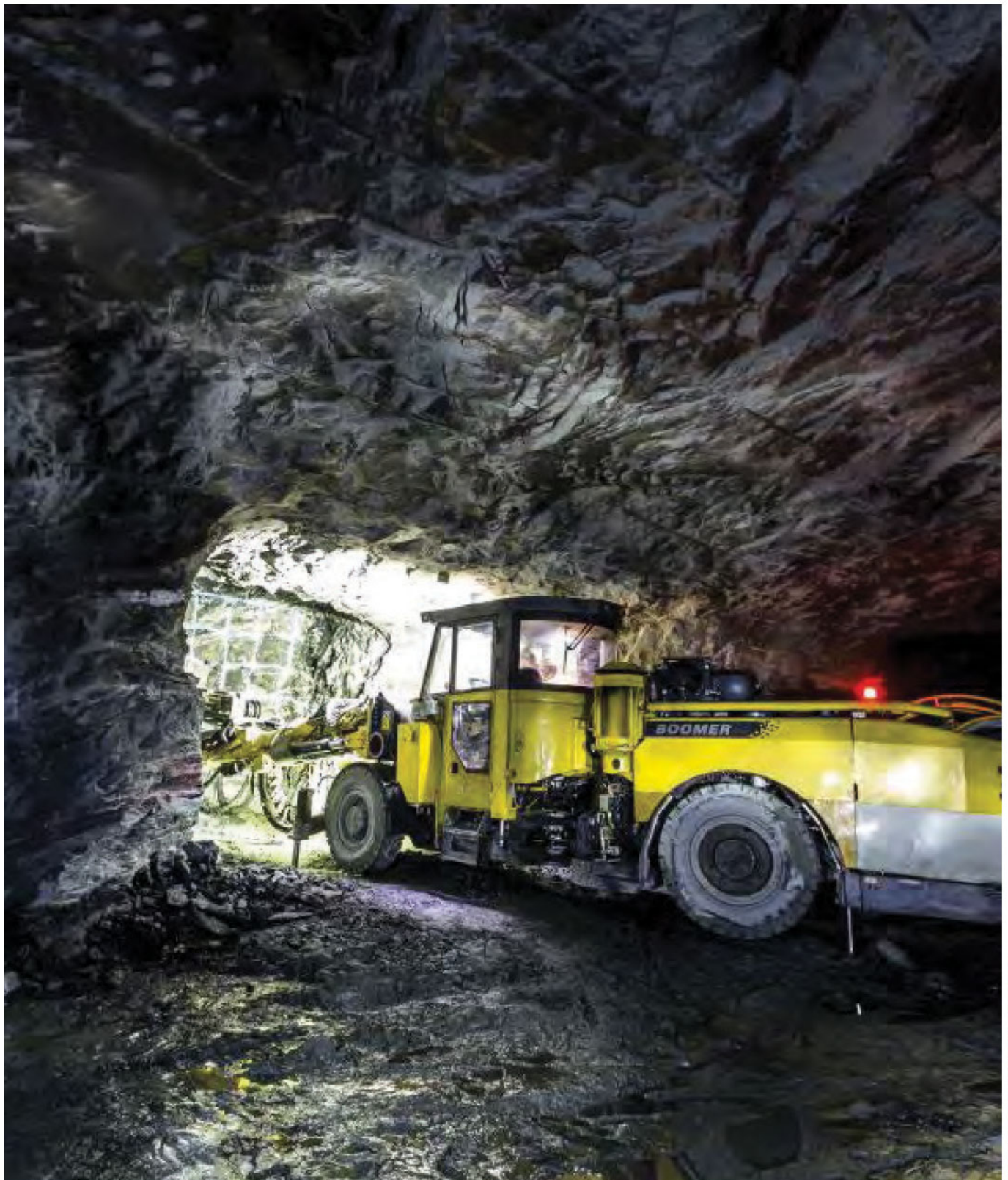
Development drilling rig underground at Serra Grande
