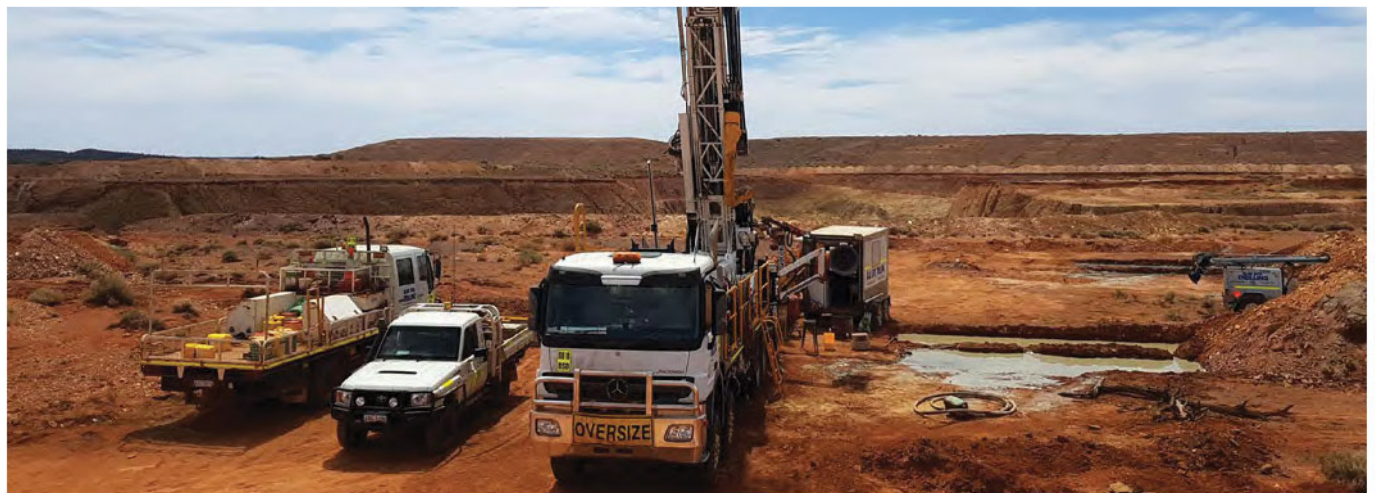
Diamond rig drilling towards the east under the Hromsky-Enigmatic pits
