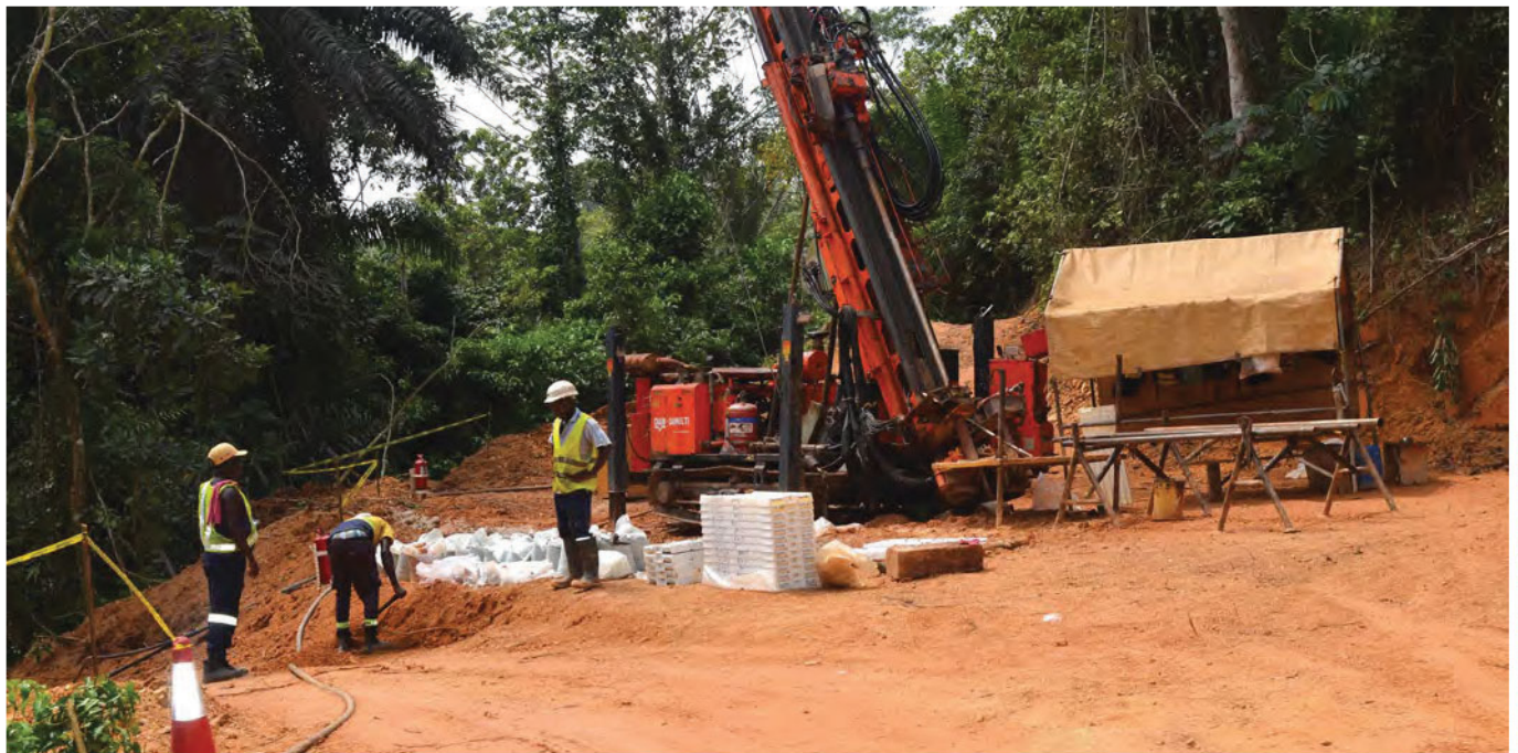
Reverse circulation exploration drilling at Iduapriem
