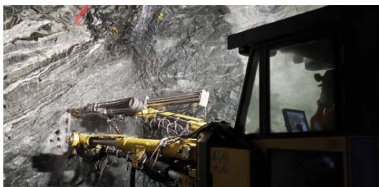
Production drill rig in action at Lamego underground
