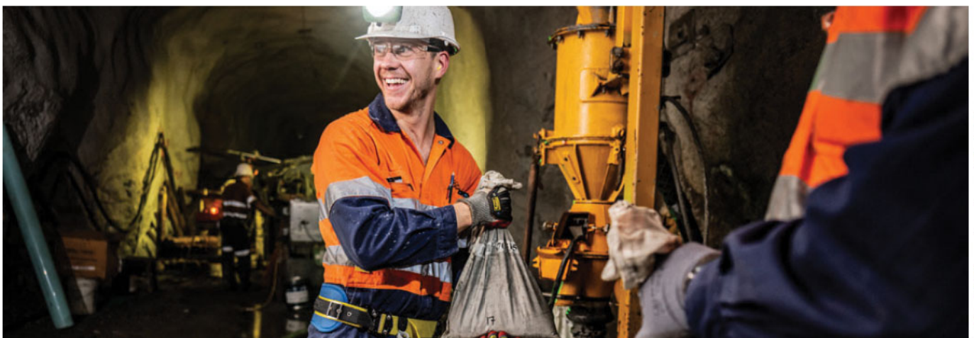
Collecting RC drilling samples underground at Sunrise Dam
