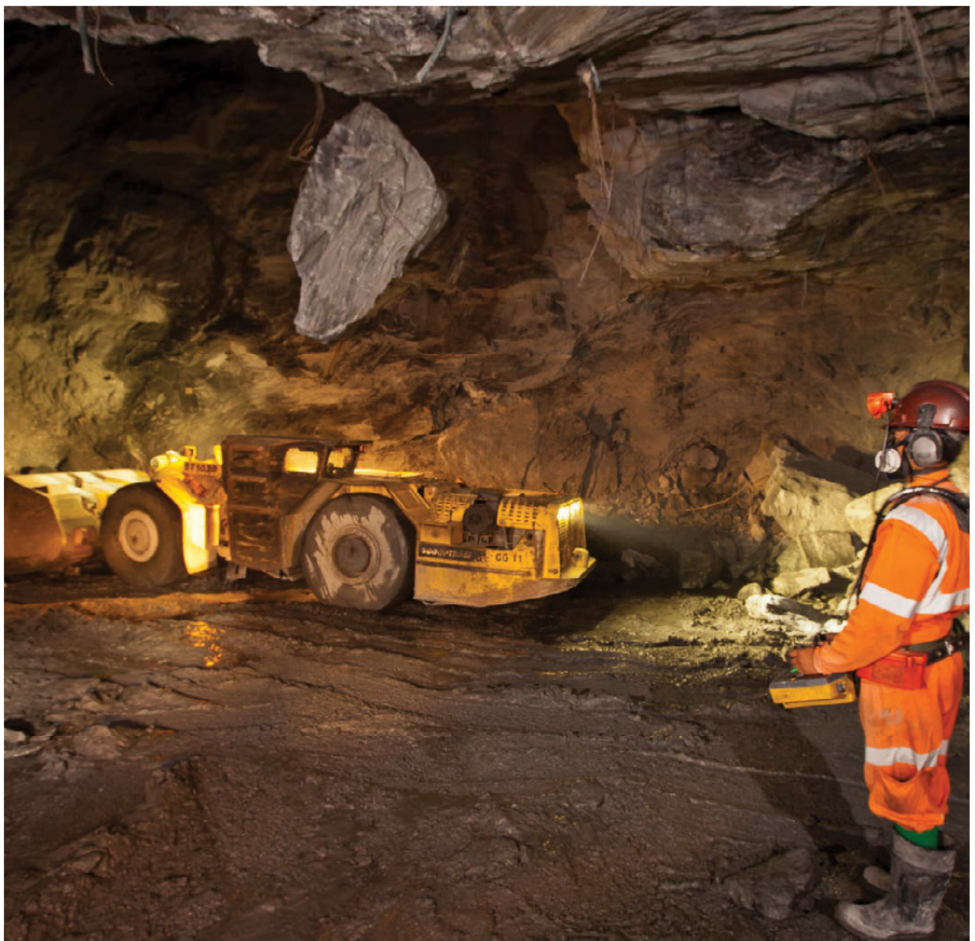
Remote operated front-end loader
