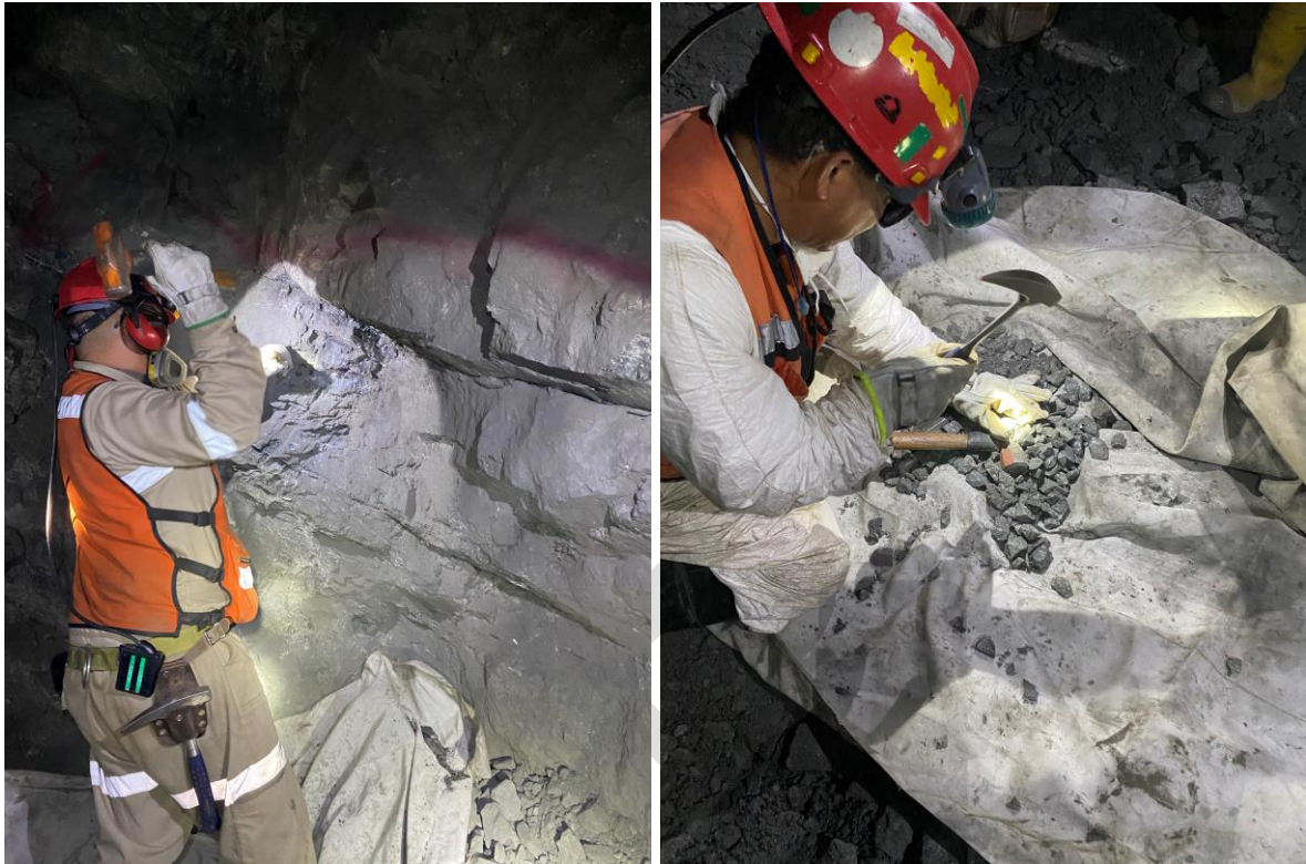
Figure 7-4: Left: Rock Sampling using Hammer and Chisel. Right: Homogenization of Fragments Size
