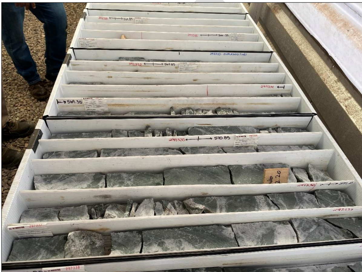
Figure 7-9: Core Boxes with Sample Marks and the Remaining Half of Core
