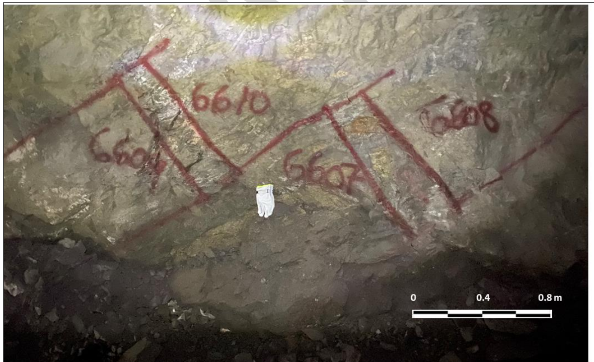
Figure 7-3: Marks Indicating Limits and Width of Samples
