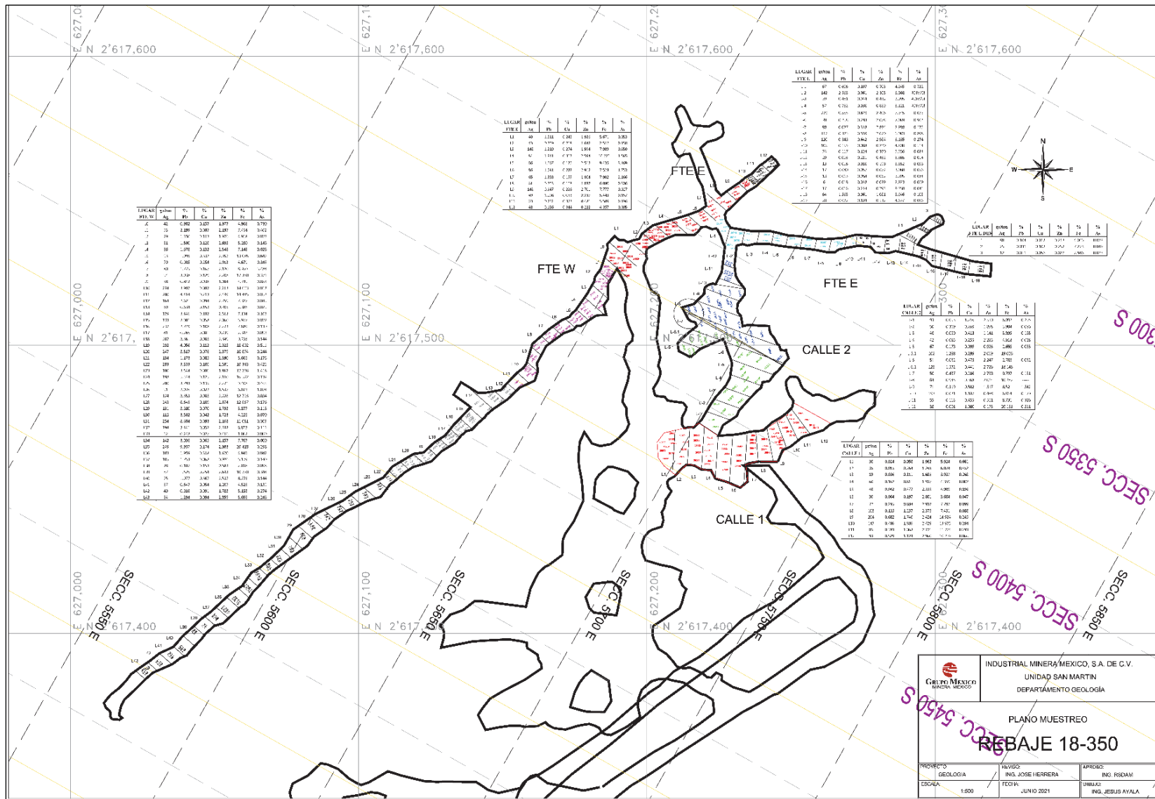
Figure 11-2: Example of Plan View of Underground Workings and Channel Sample Lines
