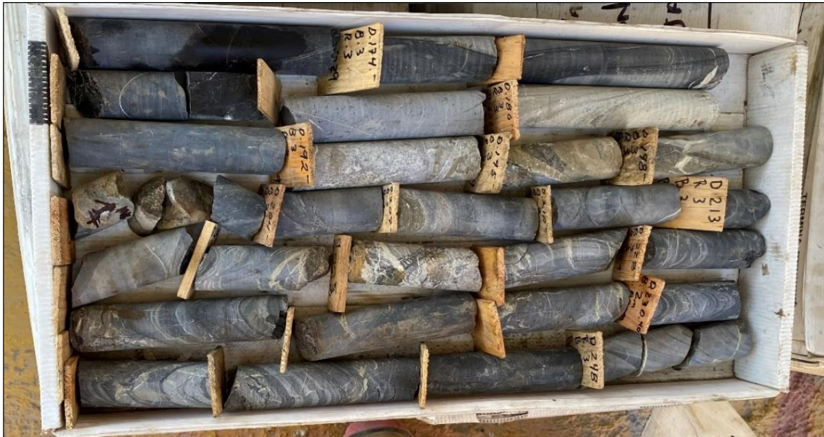
Figure 7.15: Pieces of Core of Non-Mineralized Drilling Intervals
