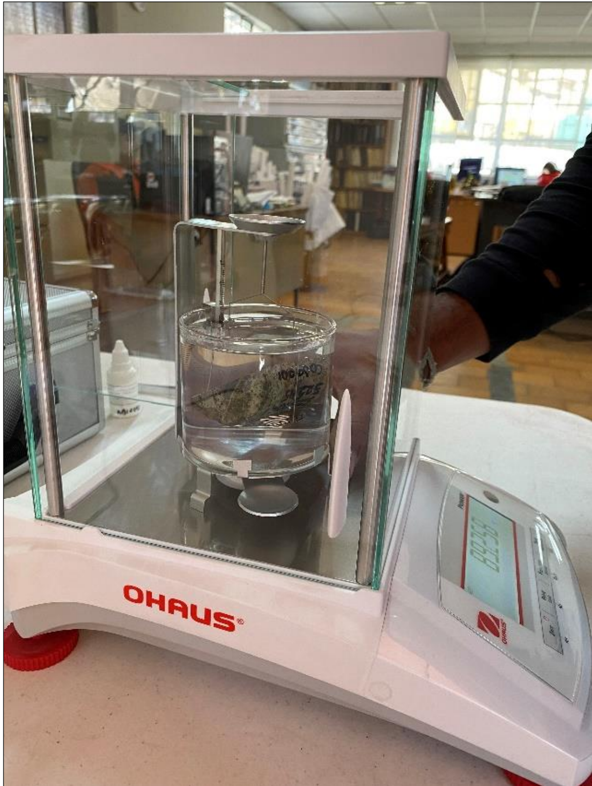
Figure 8.5: Weighting of the Sample Submerged in Water
