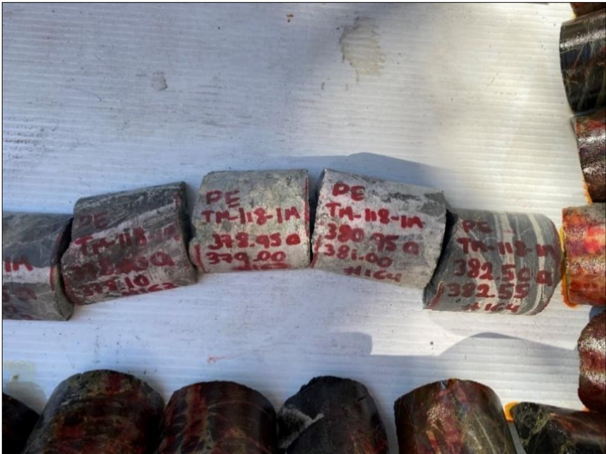
Figure 8.2: Core Samples Selected for Specific Gravity Testing
