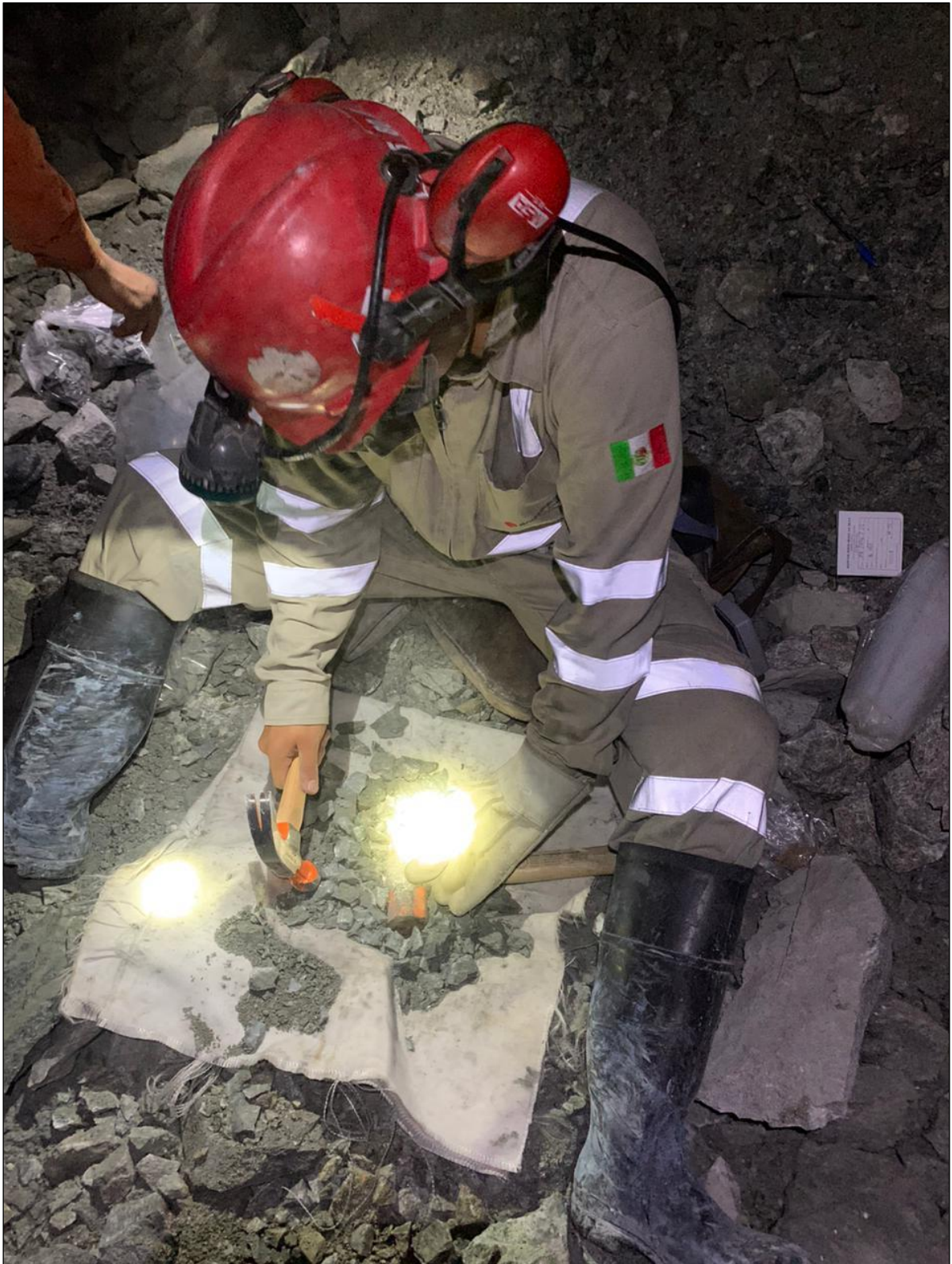
Figure 7-5: Homogenization Process of Sample Particle Size
