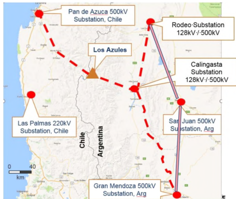
Figure 21-1: Preliminary summary of Bi-National possibilities for a power connection to Los Azules from Chile and Argentina
