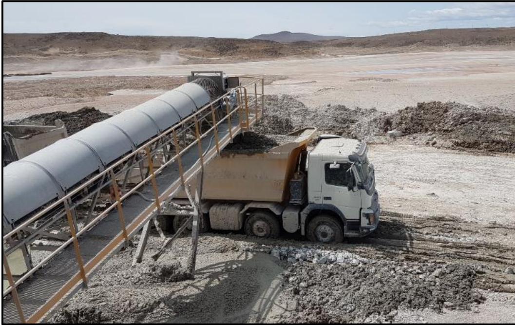
Figure 15-8 – PRA Transfer of Dewatered Tailings to Haul Trucks
