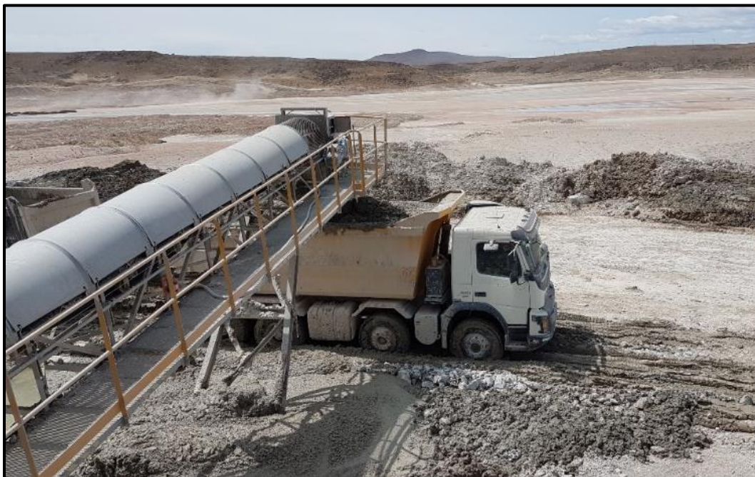
Figure 14-14 – PRA Transfer of Dewatered Tailings to Haul Trucks
