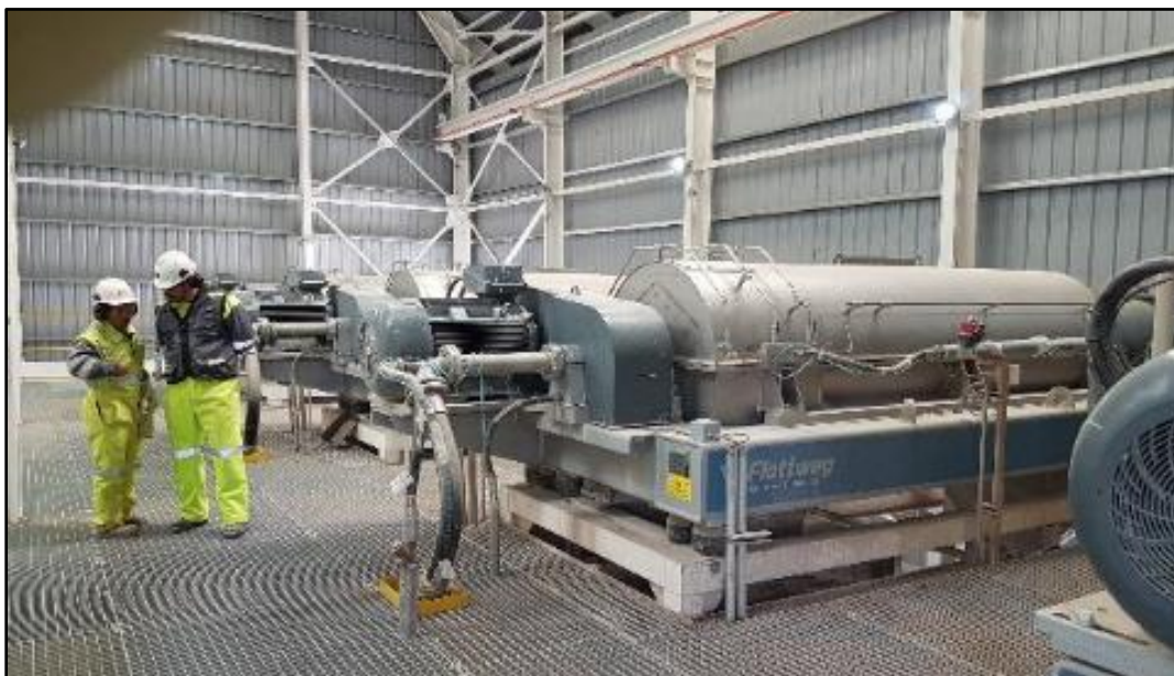
Figure 15-7 – PRA Tailings Dewatering Centrifuges
