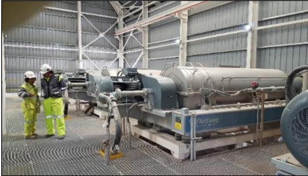
Figure 14-13 – PRA Tailings Dewatering Centrifuges
