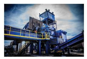
The process of shredding, which was developed in the late 1950s, allows for whole cars, appliances, and other end-of-life products
