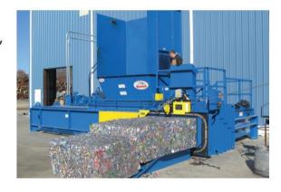
Typically, deliveries at a scrapyard will be weighed on a scale upon arrival and will then be moved, sorted, and processed using equipment such as forklifts, trucks, and cranes for transport, as well as balers, shears, wire choppers,
